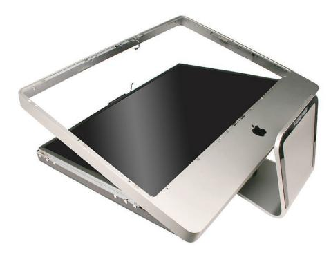
5. Replace the twelve screws around the bezel. The two longer screws (30mm) attach to the bezel along the bottom of the panel, on the right and left side of the Apple logo. The four medium length screws (19mm) attach above and below the optical drive on the right side, and on either side of the 30mm screws. The six shorter screws (15mm) attach around the top, and left side.
